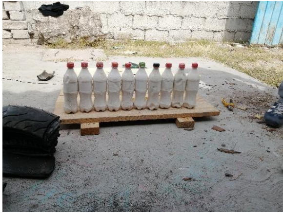
Fig. 3. The filling and compacting of the marble powder inside the PET bottles is carried out. Source: Photograph taken by the team.
