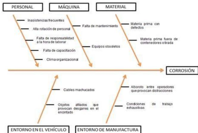
Fig. 7 Cause-effect diagram
