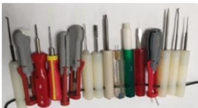
Fig. 3. Pikes that are used depending on the type of connector
